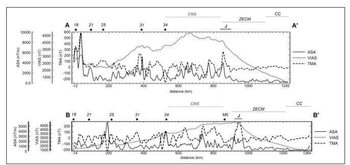
Figure 5 – Magnetic profiles A-A' and B-B' in order to illustrate the distribution on anomalies and the filtered data (ASA and VIAS) regarding the total magnetic anomaly (TMA). Location of the Cretaceous Normal Superchron (CNS), between M0 and 34 chrons. Both profiles and also the Zone of exhumed mantle (ZECM), J (J Anomaly) and CC (continental crust) were located on Figure 4. 18, 21, 25, 31, 34 are chrons locations, adapted from Muller et al. (1997).
